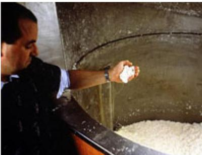
Paper pulp, in the form of sheets, is mixed with water. Then, ingredients are added to the pulp to give the paper the desired qualities for its future use:
